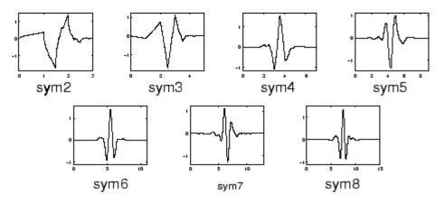
You can obtain a survey of the main properties of this family by typing waveinfo('sym') from the MATLAB command line. See "Symlet Wavelets: symN" in the *Wavelet Toolbox User's Guide* for more detail.
