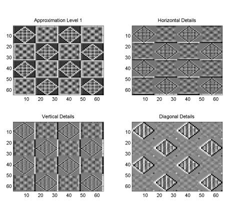
You see that the wavelet details are sensitive to particular orientations in the input image. The approximation coefficients are a lowpass approximation to the original image.
