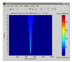
The preceding figure was modified with text labels to explicitly show which colors indicate large and small CWT coefficients.
