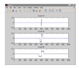
The cone of influence depends on the wavelet. You can find and plot the cone of influence for a specific wavelet with conofinf.
