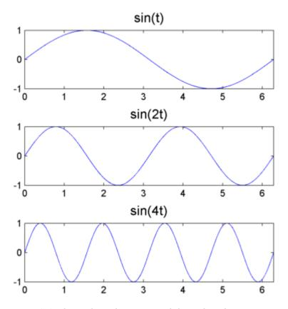
In sin(at), the scale is the inverse of the radian frequency, a.
