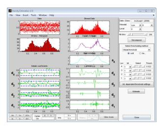
You can see that the estimation process delivers a very irregular resulting density. The density estimate (in yellow) is the normalized sum of the signals located below it: the approximation a4 and the reconstructed details after coefficient thresholding.
