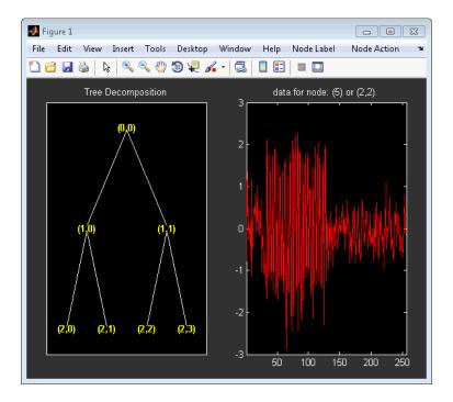
The wavelet packet transform of a 2-D image yields a quarternary wavelet packet tree. Load an example image. Use the biorthogonal B-spline wavelet with 3 vanishing moments in the reconstruction wavelet and 5 vanishing moments in the decomposition wavelet. Plot the resulting quartenary wavelet packet tree.
