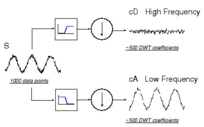
Here is our schematic diagram with real signals inserted into it.
