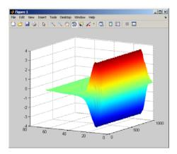
The final example constructs a signal consisting of both abrupt transitions and smooth oscillations. The signal is a 4-Hz sinusoid with two introduced discontinuities.
