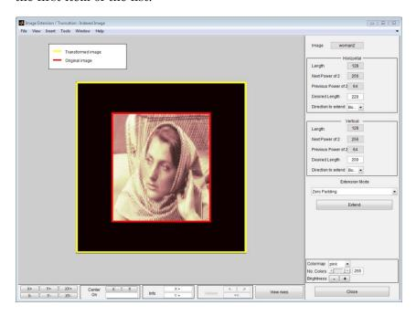
The tool displays the original image delimited by a red box and the transformed image delimited by a yellow box. The image has been extended by zero padding. The right part of the window allows you to control the parameters of the extension/truncation process for the vertical and horizontal directions, respectively. The possibilities are similar to the one-dimensional ones described in "One-Dimensional Extension" on page 2-32.
