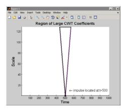
This region is referred to as the *cone of influence* of the point *t*=500 for the Haar wavelet. For a given point, the cone of influence shows you which CWT coefficients are affected by the signal value at that point.
