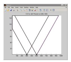
Look at point 400 for scale 20. At that scale, you can see that neither cone of influence overlaps the point 400. Therefore, you can expect that the CWT coefficient will be zero at that point and scale. The signal is only nonzero at two values, 300 and 500, and neither cone of influence for those values includes the point 400 at scale 20. You can confirm this by entering:
