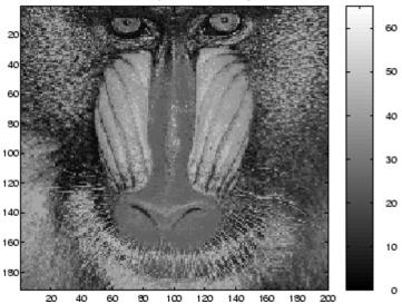
The color bar of the converted image is now linear and has a smooth transition from dark to light. The image is now suitable for wavelet decomposition.
