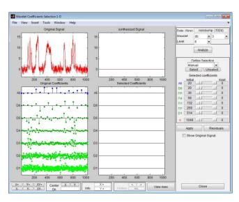
Select 16 coefficients individually by double clicking each of them using the left mouse button. The color of selected coefficients switches from green to yellow for the details and from blue to yellow for the approximation, which appear on the left of the window and appear in yellow on the middle part. Click the **Apply** button.
