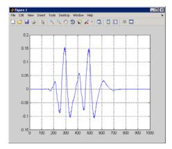
In the preceding example, the CWT coefficients became large in the vicinity of an abrupt change in the signal. This ability to detect discontinuities is a strength of the wavelet transform. The preceding example also demonstrated that the CWT coefficients localize the discontinuity best at small scales. At small scales, the small support of the wavelet ensures that the singularity only affects a small set of wavelet coefficients.
