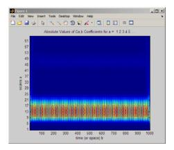
Note that the CWT coefficients are large in absolute value around scales 9 to 21. You can find the pseudo-frequencies corresponding to these scales using the command:
