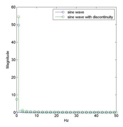
There is minimal difference in the magnitudes of the Fourier coefficients. Because the discrete Fourier basis vectors have support over the entire time interval, the discrete Fourier transform does not detect the discontinuity as efficiently as the wavelet transform.
