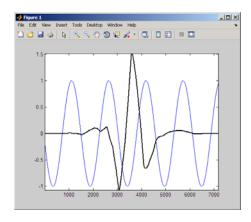
The following figure shows the product of the shifted wavelet and the sinusoid.
