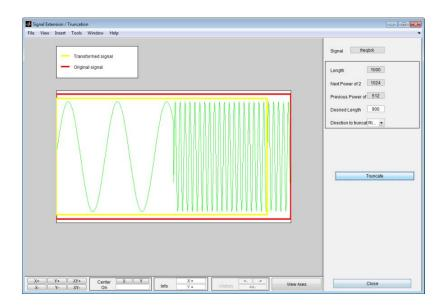
The tool displays the original signal delimited by a red box and the truncated signal delimited by a yellow box. The signal has been truncated by deleting 100 values on the right side.
