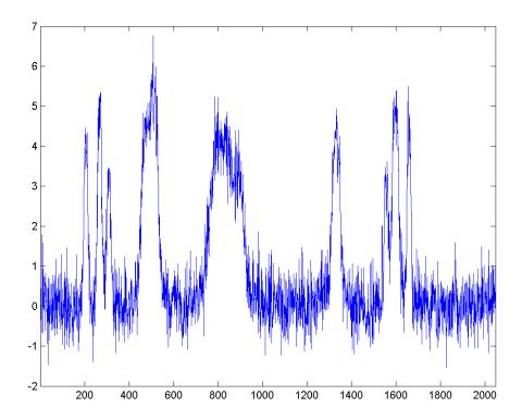
Denoise the signal down to level 3 using the Daubechies least asymmetric wavelet with 4 vanishing moments. Use the universal threshold selection rule of Donoho and Johnstone with soft thresholding based on the DWT coefficients at level 1. Use the periodization signal extension mode — <code>dwtmode('per')</code>. Plot the result along with the reference signal for comparision.
