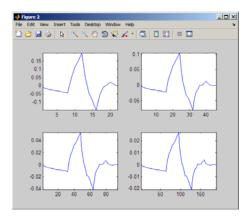
The curve begins to look progressively more like the db2 wavelet. This means that the wavelet's shape is determined entirely by the coefficients of the reconstruction filters.
