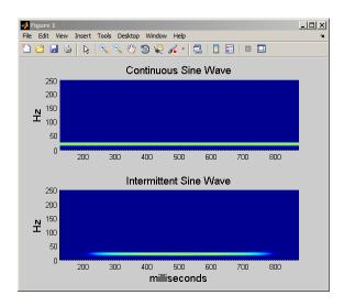
By using the STFT, you can see that the intermittent sine wave begins near 250 msec and ends around 750 msec. Additionally, you can see that the signal's energy is concentrated around 20 Hz.
