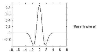
You can obtain a survey of the main properties of this family by typing waveinfo('mexh') from the MATLAB command line. See "Mexican Hat Wavelet: mexh" in the *Wavelet Toolbox User's Guide* for more information.
