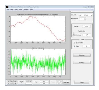
The synthesized signal clearly exhibits a stronger low-frequency component and has locally a less irregular behavior. These properties can be investigated by clicking the **Statistics** button.
