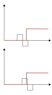
In the top figure, the wavelet has just begun to overlap with the unity portion of the unit step. In this case, the CWT coefficients are negative, but not as large in absolute value as those obtained at position B. In the bottom figure, the wavelet has shifted past position B and the positive deflection of the wavelet begins to contribute to the integral. The CWT coefficients are still negative, but not as large in absolute value as those obtained at position B.
