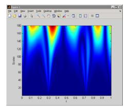
Note that the CWT detects both the abrupt transitions and oscillations in the signal. The abrupt transitions affect the CWT coefficients at all scales and clearly separate themselves from smoother signal features at small scales. On the other hand, the maxima and minima of the 2–Hz sinusoid are evident in the CWT coefficients at large scales and not apparent at small scales.
