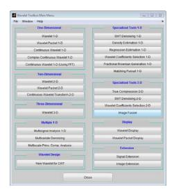
Click the **Density Estimation 1-D** menu item. The discrete wavelet analysis tool for one-dimensional density estimation appears.
