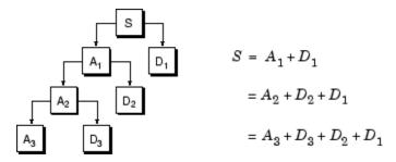
In wavelet packet analysis, the details as well as the approximations can be split.
