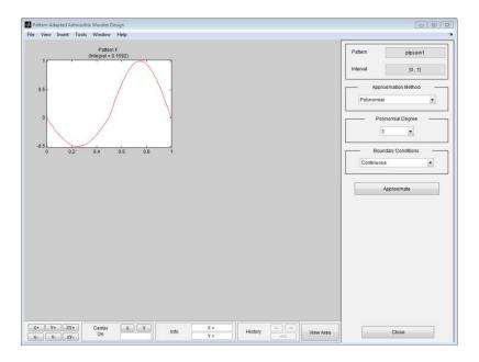
The selected pattern denoted by F is defined on the interval [0,1] and is of integral 0.1592. It is not a wavelet, but it is a good candidate because it oscillates like a wavelet.
