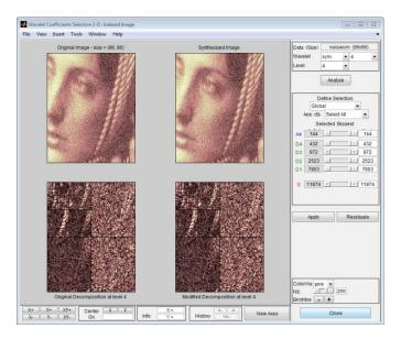
The tool displays its wavelet decomposition below the original image (on the left). The selected coefficients are displayed in the middle of the window, below the synthesized image (which, at this step, is the same since all the wavelet coefficients are kept). There are 11874 coefficients, a little bit more than the original image number of pixels, which is 96x96 = 9216.
