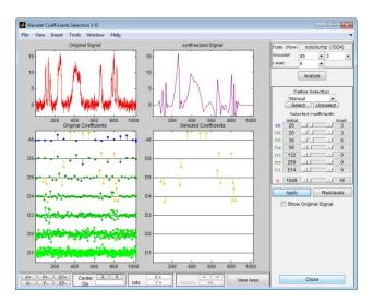
You can deselect the currently selected coefficients by double clicking each of them. Another way to select or deselect a set of coefficients is to use the selection box. Drag a rubber band box (hold down the left mouse button) over a portion of the coefficient axes (original or selected) containing all the currently selected coefficients. Click the **Unselect** button located on the right of the window. Click the **Apply** button. The tool displays the null signal again.
