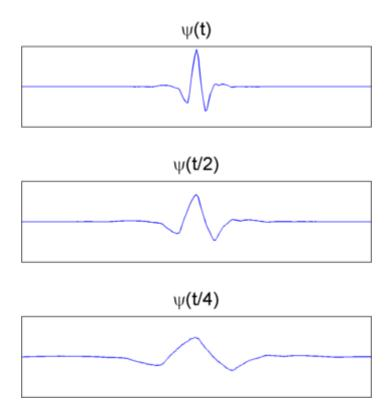
This general inverse relationship between scale and frequency holds for signals in general. See "CWT as a Filtering Technique" on page 1-26 and "Scale and Frequency" on page 1-23 for more information on the relationship between scale and frequency.
